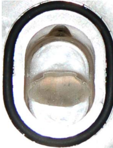
Figure 6-29: TS7 Silver Insert Post-Irradiation
