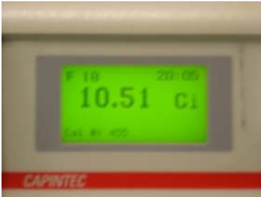
Figure 6-32: 10.5 Ci of ^{18}\text{F} in Dose Calibrator
